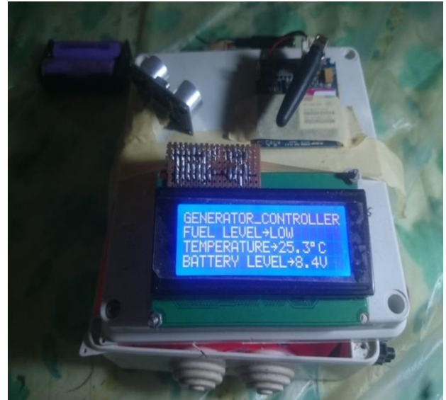
Figure 13: Status of Generator of when Temperature below Rated Maximum Value and Fuel Level is Low
