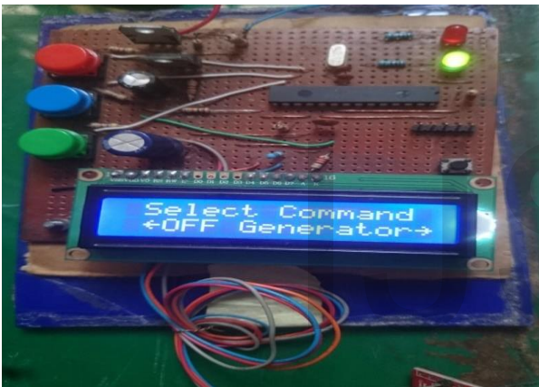
Figure 11: Menu to Switch OFF the Generator
